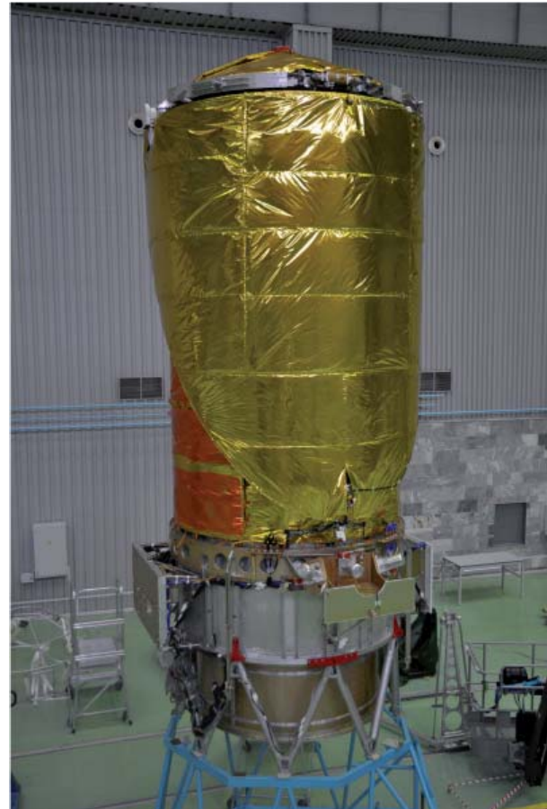
Fig. 2 The T-170M telescope at the Lavochkin Science & Technology Association after vibration-vacuum tests.
