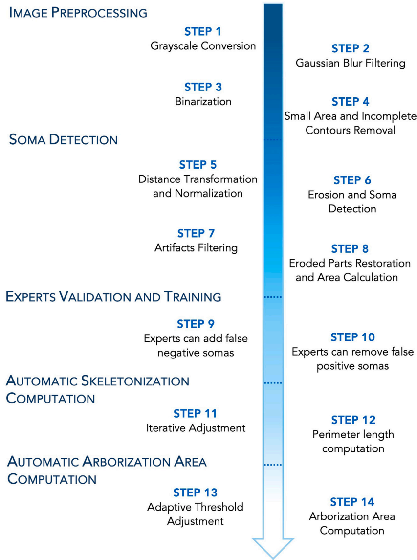
Fig. 1. System Flowchart. First, the image undergoes preprocessing. Next, soma detection is performed, allowing the user to add or remove somas if needed. Then, the skeletonization results are computed and presented to the user. Finally, the arborization area computations are displayed.
