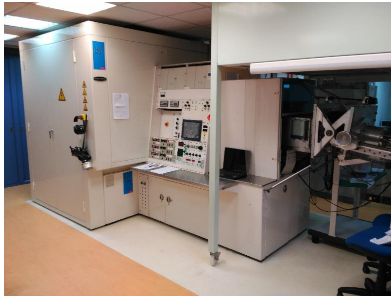
Figure 2-5 Ion implantation system at CAI of physical techniques from UCM.
