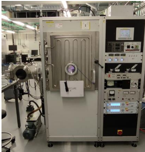
Figure 2-2 RF sputtering system at PV-Lab (EPFL) used to deposit ITO:H
