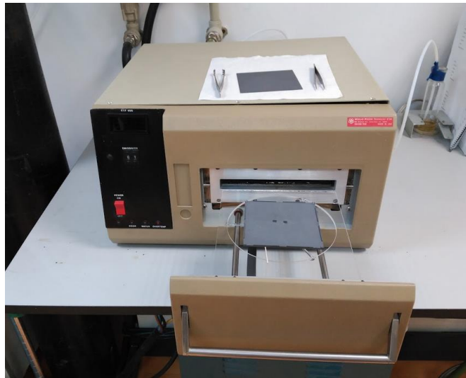
Figure 2-7 Rapid thermal annealing system employed to activate the impurities introduced during the ion implantation process.
