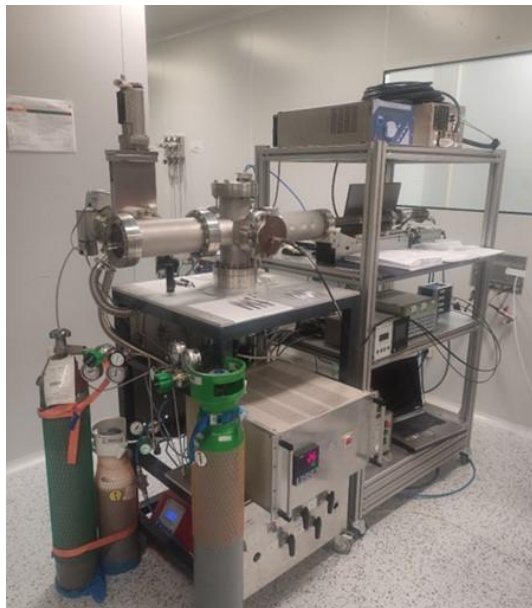
Figure 2-4 Photograph of the high-pressure sputtering system used during this thesis to deposit ITO and TiO x films.
