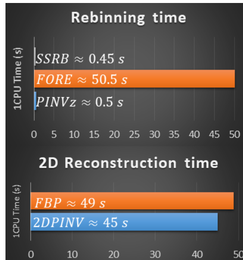
Figure 73: Computational times for the different methods for clinical data acquired in a Biograph TPTV scanner. Input sinograms were 336 \times 336 \times 559 bins. Reconstructed images were 255 \times 255 \times 109 voxels.
