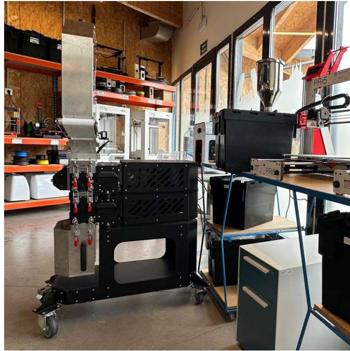
Figure A.2: 3devo's shredder and dryer. Image provided by Gonzalo Alonso García
