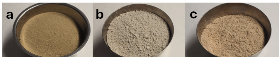
Fig. 2. Raw materials applied in this study: (a) natural expansive soil, (b) cement kiln dust from the factory in Carboneras (CKDC), (c) cement kiln dust from the factory in Villaluenga de Sagra (CKDVS).
