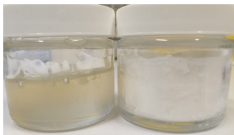
Figure 4. Crude PPP1500 (left) and PPP3000 (right) polymers after their synthesis and freeze-dried.
