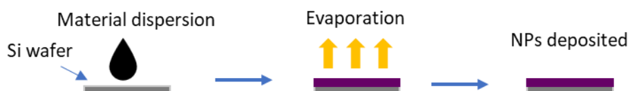
Figure 2.12. Deposition method using drop casting.
