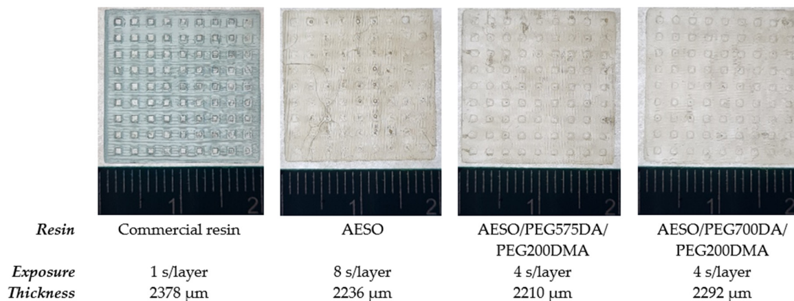
Figure 7. Comparison of four 3D-printed samples, using the same shape and different resin mixtures. Images taken using a cell-phone camera at 3 \times magnification, near a measuring ruler expressed in centimeters.
