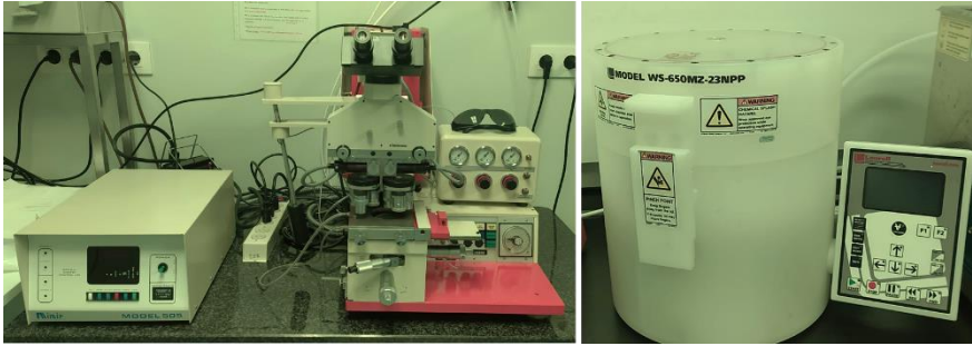
Figure 2.2. (left) Photograph of the alignment and exposure system. (right) Photograph of spinner system
