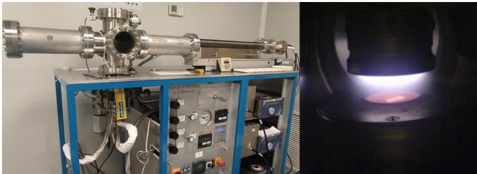
Figure 2.1. (left) Sputtering chamber (right) oxygen plasma formed at the sputtering target.
