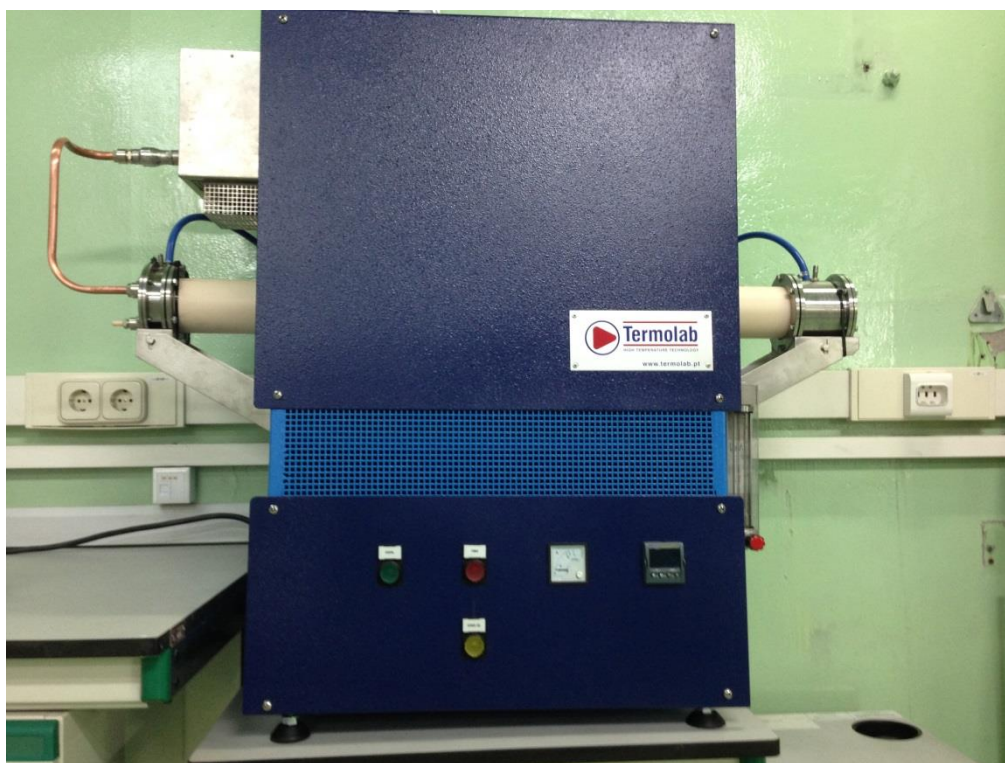
Figure 3.3. Tubular horizontal furnace TH1700 used in this thesis for sintering ATF pellets.
