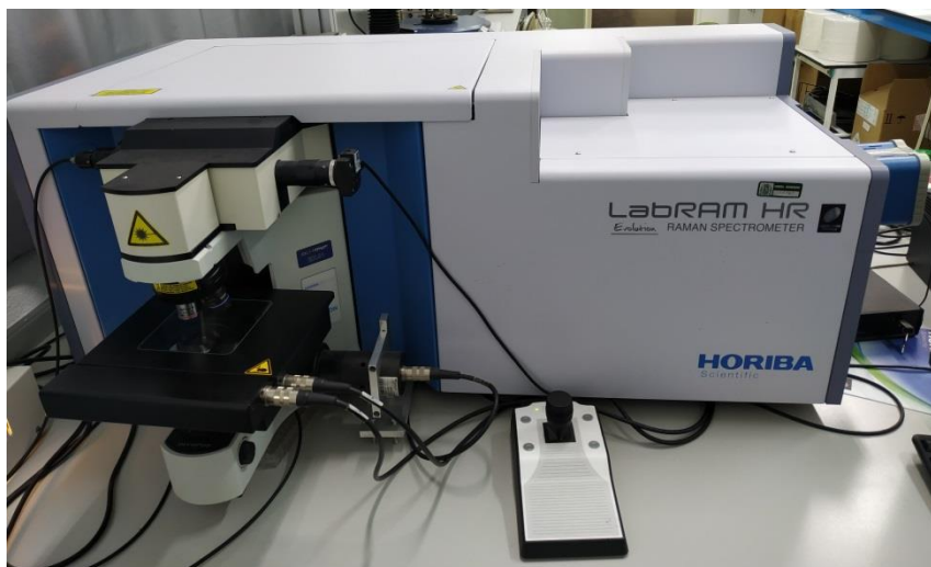
Figure 3.4. General view of the HORIBA LabRAM HR Evolution spectrometer.
