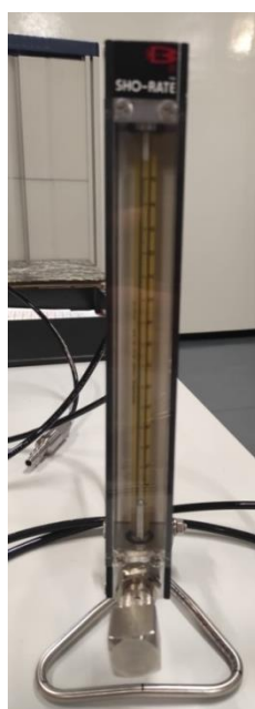
Figure 3.19. Sho-Rate flow meter used to control the gas flow during the oxidation experiments at JRC.
