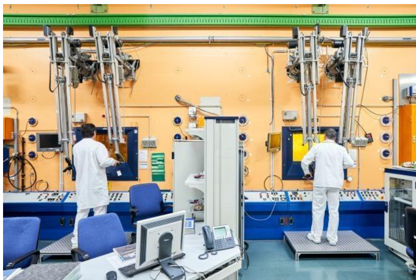
Figure 3.13. External view of two hot cells available at JRC facilities, with two workers holding the telemanipulators for nuclear fuel handling. Image taken from [20].
