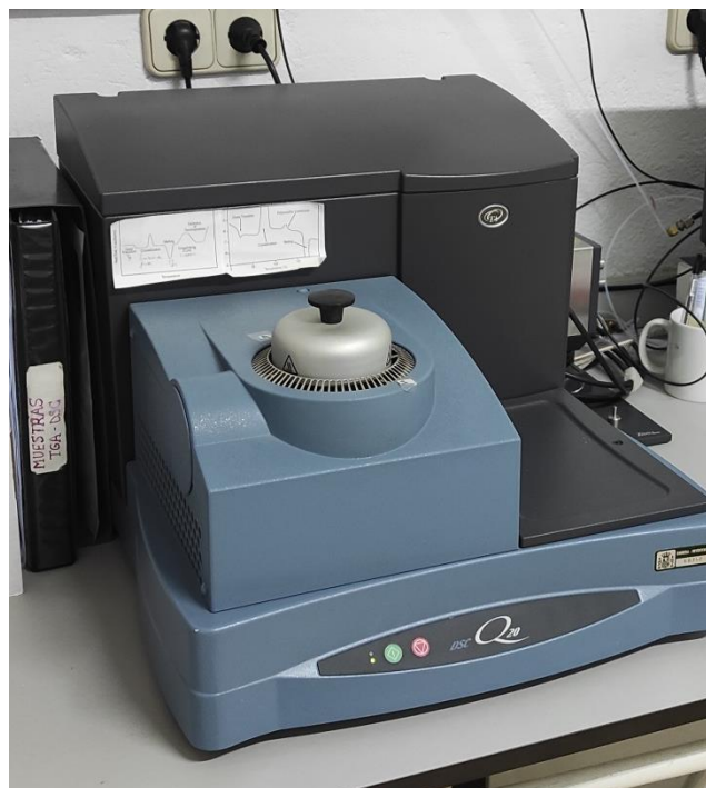
Figure 3.7. TA Instruments DSC Q20 instrument.
