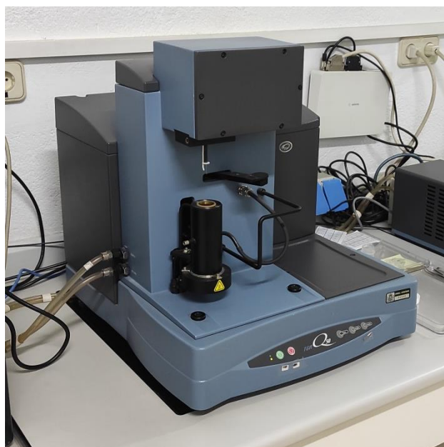
Figure 3.6. TA Instruments TGA Q50 thermobalance for thermogravimetric experiments.
