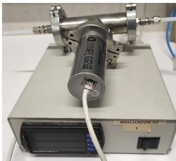
Figure 3.17. Zirconia oxygen sensor and associated instrument, where the oxygen concentration (in ppm) is displayed.
