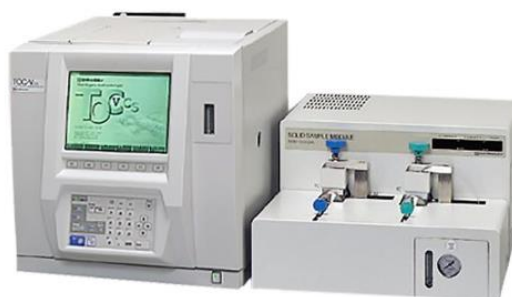
Figure 6.10. TOC-V CSH analyser (left) and SSM 5000 solid sampler (right).
