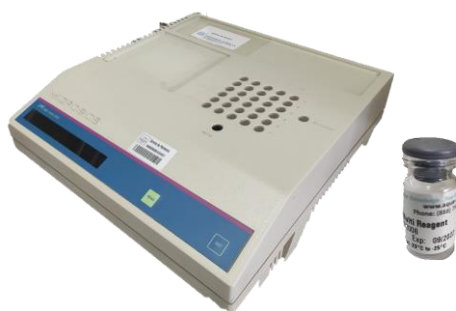
Figure 6.11. Microtox® M500 Analyzer (Microbics Corporation, USA) (left) and Vibrio fischeri bacteria (right).
