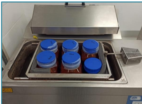
Figure 9.2. Experimental device for treatment of soils P1, P2 and P3.
