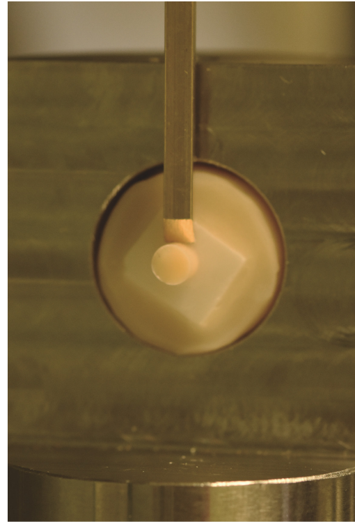
Fig. 1. Specimen prepared for SBS test placed on the testing machine.
