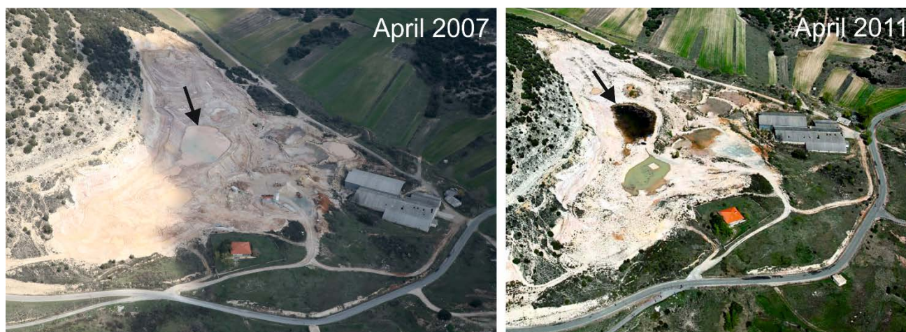
Figure 3. The 2007 image shows the quarry closure and stabilization works, regrading platforms and sediment ponds construction (the black arrow points to the main one, which is the one visible at Figure 2F). As it can be seen in the 2011 image, four years later, the surface had not recovered any soils or vegetation.
