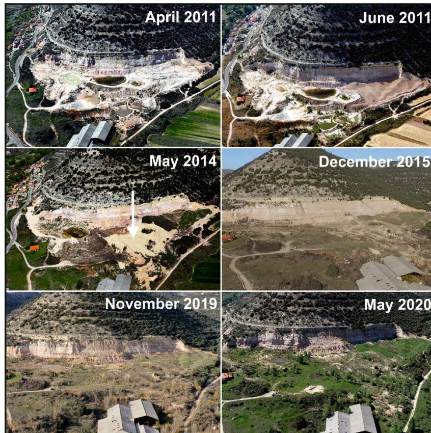
Figure 7. Comparison of oblique aerial photos of the Somolinos quarry from April 2011 (before restoration) to May 2020. Notice the 1-ha surface restored in June 2011. At the May 2014 photo, the lighter colours (white arrow) are the central area left without manure amendment. Photos by Paisajes Españoles (2011, 2014), David Gutiérrez (DGDRONE, 2015, 2020) and Javier Melero (2019).
