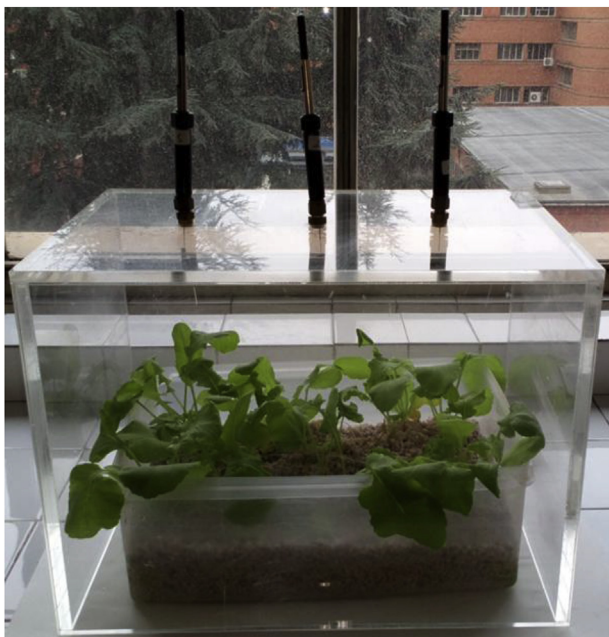
Fig. 1. Experimental set-up employed for extracting volatile selenium compounds released from plants exposed to Cs-SeNPs by HS-SMPE.
