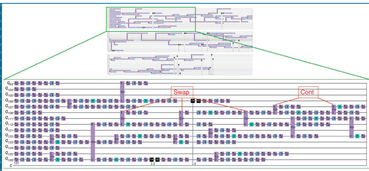
FIGURE 4. Measurement-based preparation of the logical |+\rangle state for the Q_1(N=8, i=3) code from Figure 2, mapped into ibm_sherbrooke topology using noise-aware compilation technique (top). The original CNOT gate was mapped using the native ECR gate and single-qubit prerotations. Partial detail (bottom).
