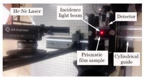
Figure 5. Experimental setup for the transmittance measurements (upper view).
