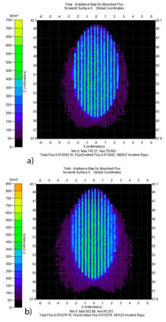
**Figure 7**. Flux loss rate obtained in tridimensional simulations of CPLG guides with curvatures of 8.00 (a) and 57.14 (b).
