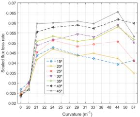
**Figure 6**. Light flux rate (rate of flux lost) scaled from 0 to 1.0 as a function of the curvature of a CPLG for several incidence angles. The graph legend shows incidence angles with regard to the prismatic film flat surface.
