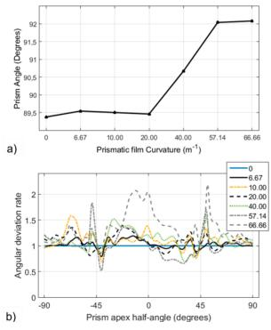
**Figure 4.** Angle  $\theta$  obtained by HT related with CPLG curvature. The graph legend shows curvatures evaluated in m<sup>-1</sup>. Global changes in prismatic angle related with Hough peaks are shown in (a) and local changes in prism half-angle in (b).
