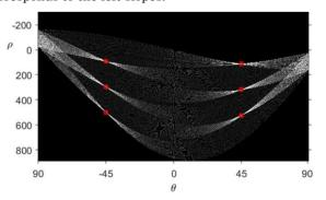
**Figure 3.** The HT of the three prisms image of prismatic film curvature of 20 m<sup>-1</sup> with Hough peak identified. The red square shows the peaks of data in the Hough matrix indicates  $\rho$  the perpendicular distance from the origin to
