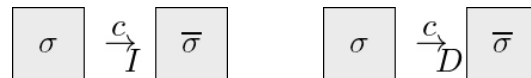
FIGURE 2.1: If the current cell is in state \sigma , then the state of the cell being c positions to the left (or to the right, respectively) will change its state to \bar{\sigma} . More specifically, c will be of the form c = 2^k , where k is a counter that will be increased by one after each time step and that we can initialize back to 0 when needed.
