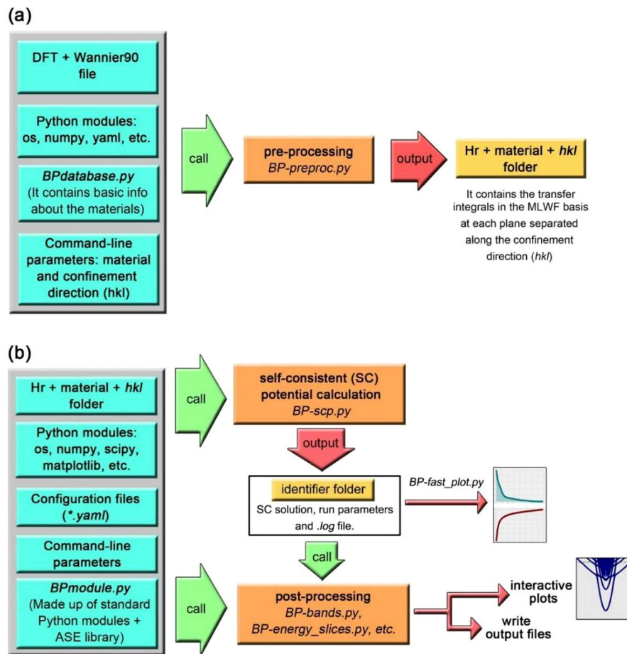
Fig. 4. Working structure of BinPo . (a) Pre-processing step. (b) Self-consistent potential energy calculation and post-processing steps.
