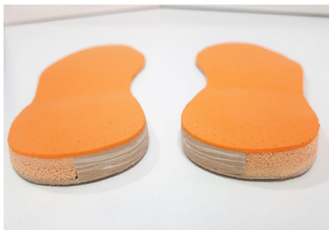
Figure 1. Novel supination orthosis made using 3 mm-thick ethylene-vinyl acetate and lateral cushioning casting filled with Poron.
