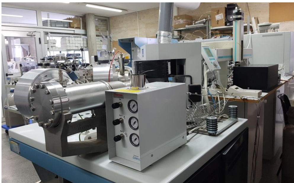
Figure 17. Thermo Finnigan MAT 253 for the analysis of isotopic composition ( ^{13}\text{C}/^{12}\text{C} ) of \text{CO}_2 ( \delta^{13}\text{C-CO}_2 ).
