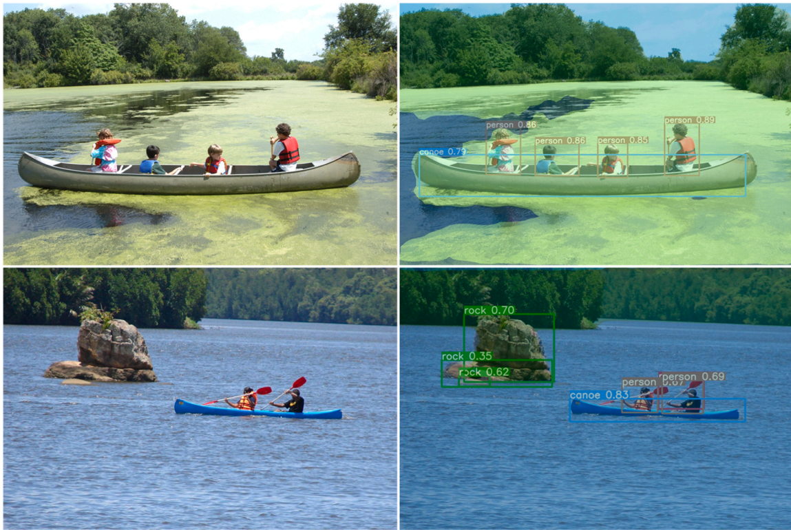
Fig. 1. Samples of the integration of object detection and semantic segmentation. The images on the left side are the RGB images, and the images on the right side are the results of the integration of object detection and semantic segmentation.
