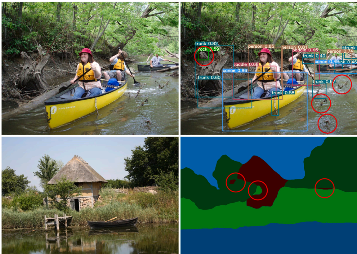
Fig. 17. Visual presentation of the suboptimal result for both object detection and semantic segmentation. The first row corresponds to the object detection result and the second row to the semantic segmentation result.
