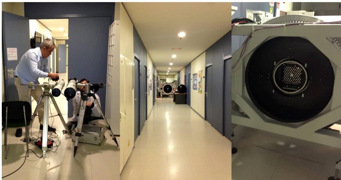
Figure 15: Positioners parameters laboratory verification set-up views. Left: Preparing telescopes, camera and CCD to register images. Center: Fiber MOS assembly at the opposite site of the corridor (18 m distance). Right: Fiber MOS minibundles back illuminated.
