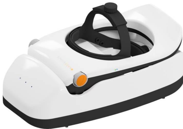
Figure 4.12 First prototype of the SimVis Gekko Dock, based on the low-speed low-cost focimeter presented in the current chapter.
