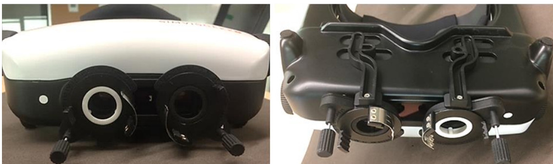
Figure 2.6 Trial frames to compensate the refractive error of the patient, attached to the SimVis Gekko modules employing magnets.
