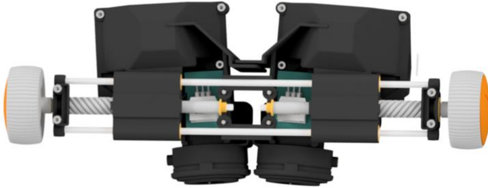
Figure 2.5 Design of the optical module with the 2.25^\circ convergence angle between channels optimized for 80 cm, and the lateral screw for the horizontal movement of the optical module to allow different interpupillary distances.
