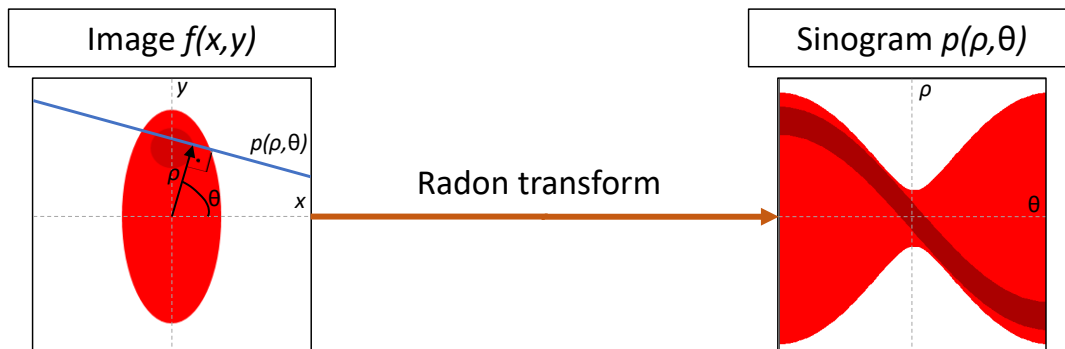
Figure 1.7: Pictorial scheme of the Radon transform. The coordinates (\rho, \theta) in the sinogram domain (right panel) are correlated with the projection at a fixed angle and radial distance in the image domain (left panel).
