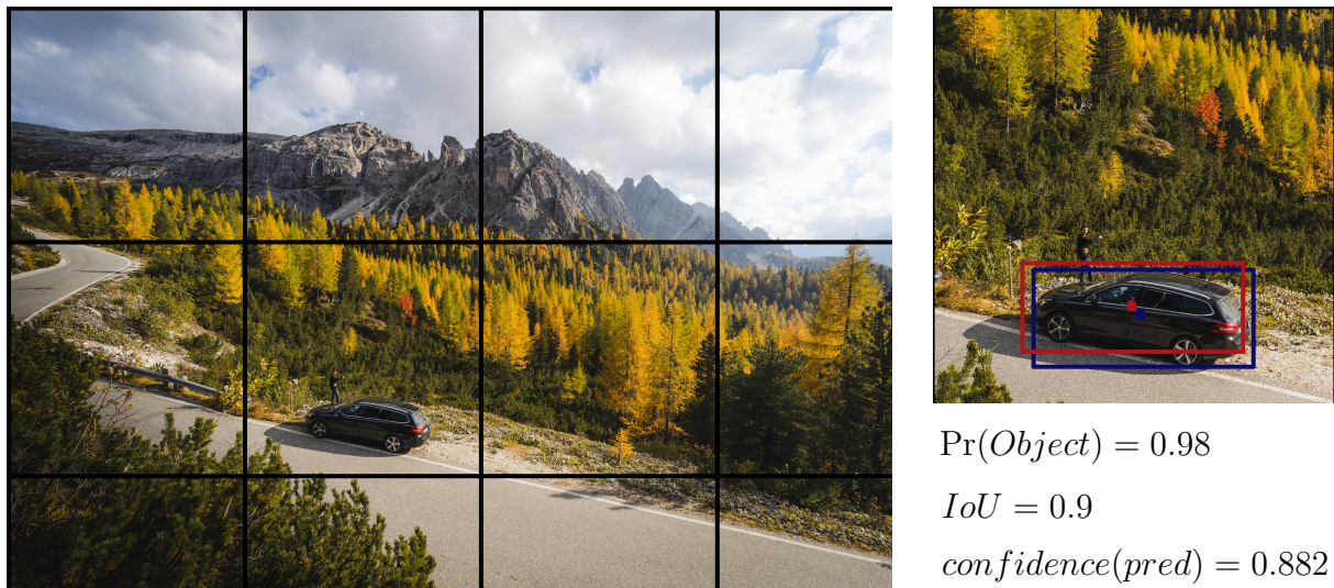
Figure 2.4: YOLO confidence score calculation. On the right, predicted bounding box (red) versus ground-truth (blue) for one of the grid squares.
