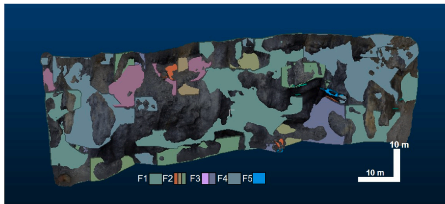
Fig. 6. Results of the FACETS analysis with the main discontinuity planes F1, F2, F3, F4, F5 obtained from the 3D point cloud.
