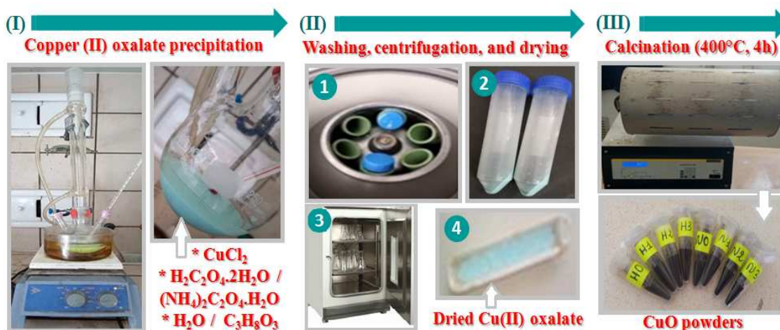
Figure 1. Illustration of the synthesis process of CuO-NPs.
