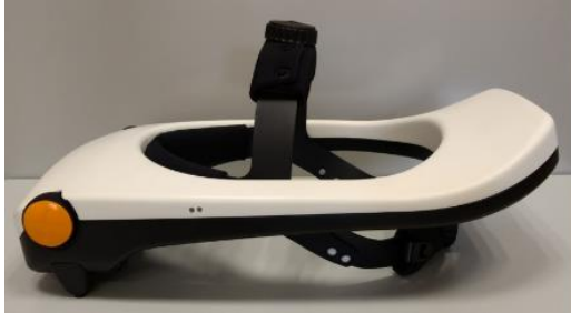
FIGURE 2.5. SimVis Gekko™, binocular, programable, portable, wireless, and wide visual field device (2EyesVision S.L).
